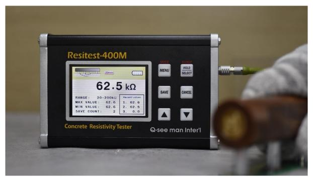
The corrosion of steel in concrete is an electro-chemical process which creates a current flow causing metal to dissolve so that it is possible to assess the probability of reinforcement corrosion by evaluating the electrical resistance of the concrete. The factor is measured in terms of resistivity and expressed in Ohm.
